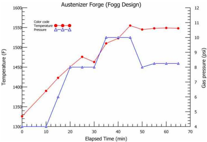
the system needed about 8.25 psi pressure to hover at 1550 F. When the door was opened (as in removing a blade for quenching), the temperature popped up to 1575 F - indicating that there must have been a reducing atmosphere in the forge. Looks promising!
