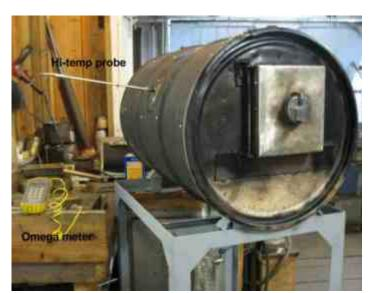
(showing temp meter & probe)
